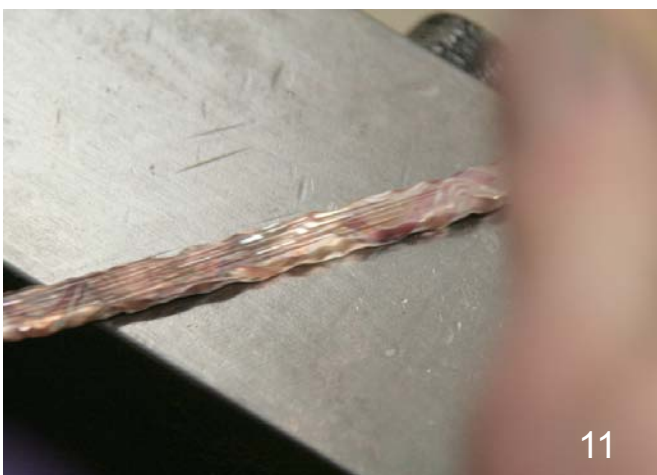
Surface hardening from wimpy blows may cause delaminations.
