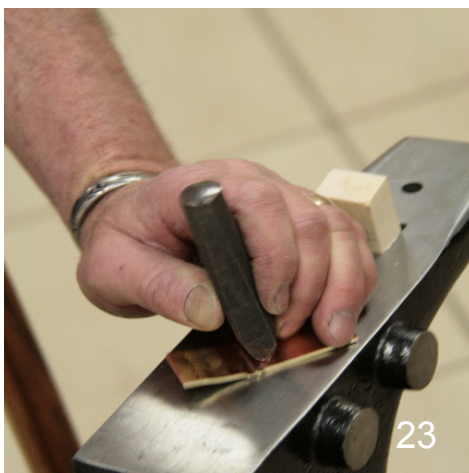
Note the wood peg in the hardy hole to soften the anvil's ring.
