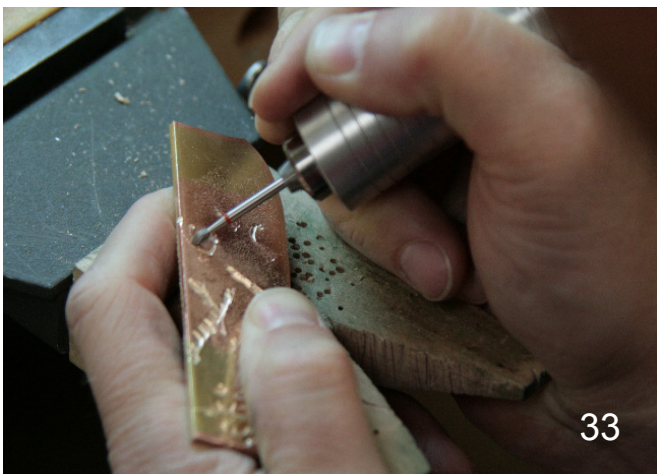
Pattern development by stock removal.
