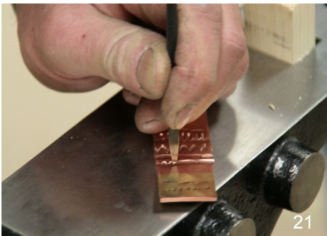
Note the punches are driven deep into the stock.
