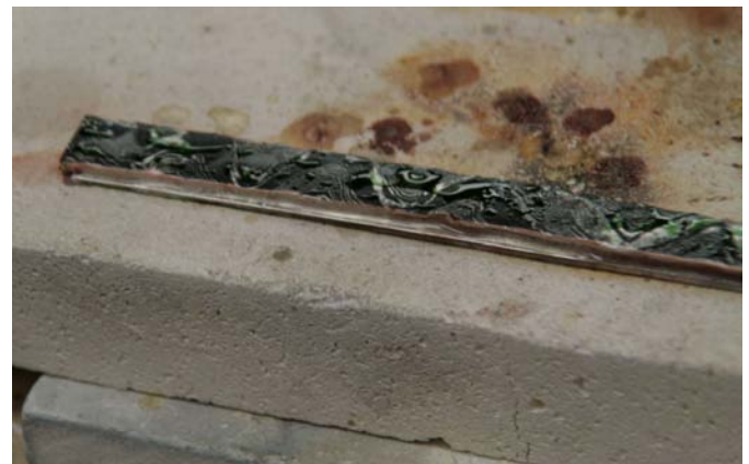
A well soldered joint.
