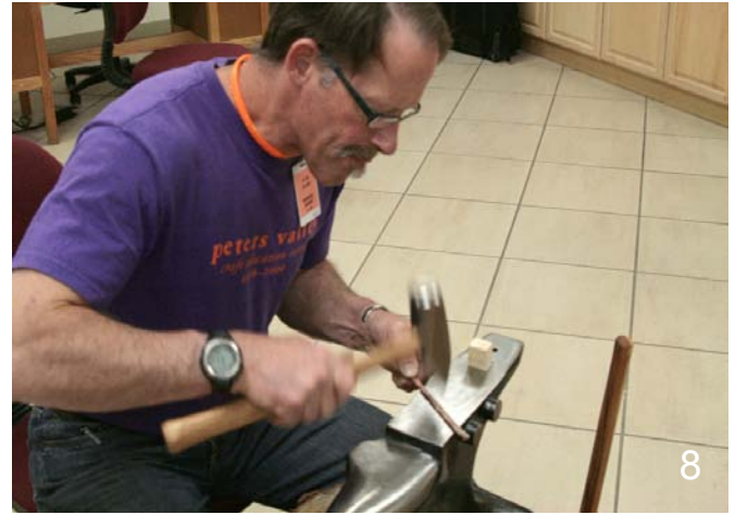
Note that these are forging hammers! Heavy hits are better than little taps.
