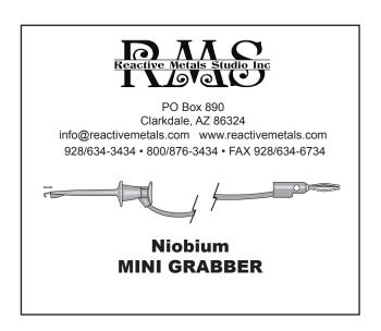
Your new Niobium MINI Grabber is the first holder produced for anodizing Niobium. The special tip is made from Niobium wire. It can be used to hold Niobium and Titanium for anodizing. It can safely be submerged up to where the lettering starts on the shaft. Above this point the stainless steel spring will be conductive which may slow the anodizing process and eventually dissolve the spring.
